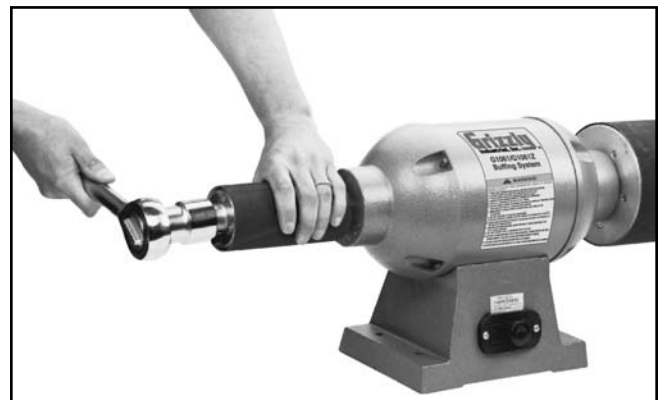
Figure 5. Sanding drum loosening/tightening procedure.
